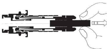
Connection can not be broken by pulling the cable or any other parts of the plug than the outer shell.
