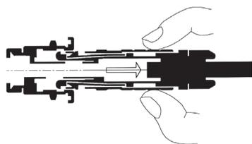
To unmate the plug from the receptacle, just pull the outer shell axially.
