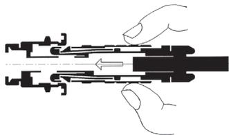
The latching of the plug into the receptacle is achieved by a simple axial push of the outer plug shell.
